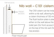
The C101 cistern can be installed within a nib wall, allowing for a cistern thickness of 130 mm. The flush button plate is placed either on the wall above the toilet pan (for front access) OR on the top of the nib wall (for top access).
