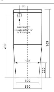
BACK ENTRY INLET OPTION: 1/2" BSP nipple approx 22mm projection from finished wall 440 0 80 150 rec \_ 150 setout recommended 80 215 (range 90-180)
