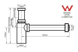
When Using the AU4040-VE Vertical Extesion
