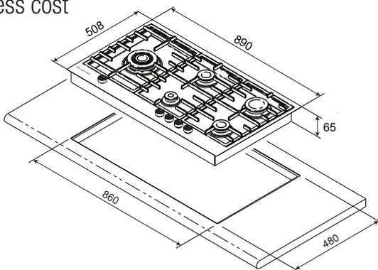
These dimensions are provided as a general guide only and should not be used for designing or constructing cabinetry or for installation.
