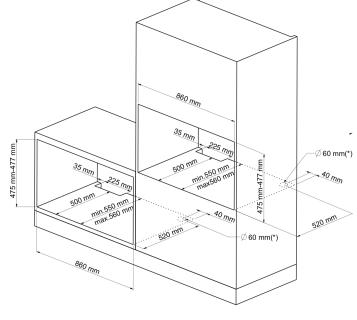
\* The 60mm hole is required for the cable to pass through
