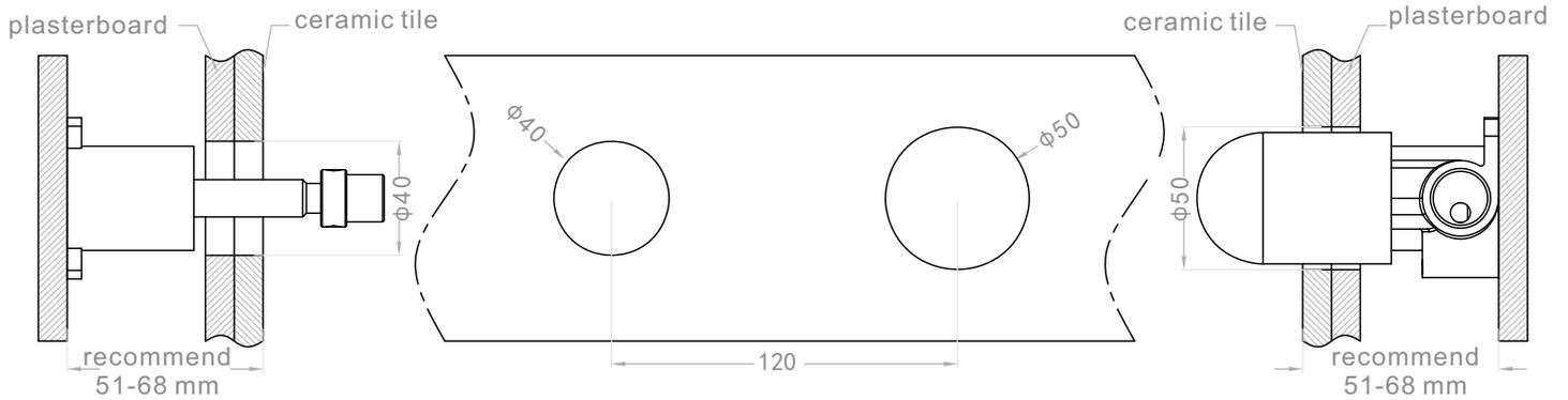
1. Fix body on noggin and ensure installation depth is 51-68mm from noggin to ceramic tile.
