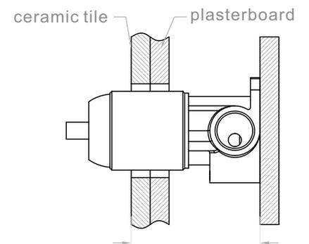
4. Remove the plastic sleeve, grub screw and water testing plug.
