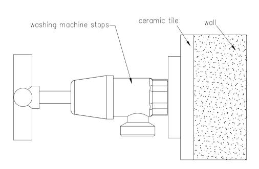
1.Put washing machine stops onto the  $G_{\overline{2}}^{1}$  outlet, and adjust the rotation angle of it.
