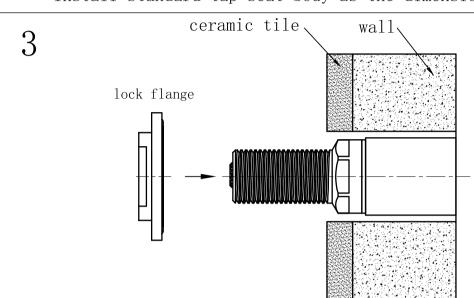
Screw lock flange tightly on the lock nut.
