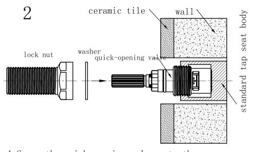
1. Screw the quick-opening valve onto the body tightly.
