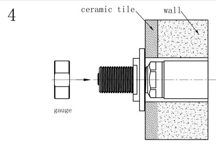
Screw gauge tightly on the lock nut.
