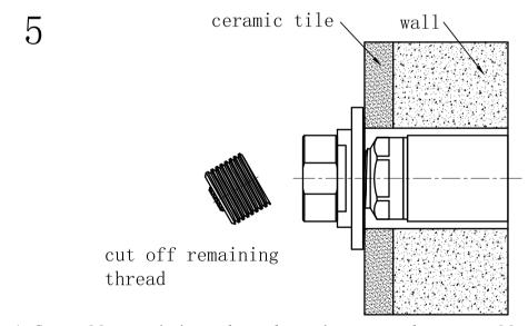
1. Cut off remaining thread against to the cut off gauge.
