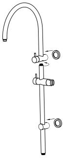
Screw shower rail into shower arm component. Tighten firmly.
