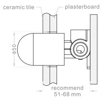
Fix body on noggin and ensure installation depth is 51-68mm from noggin to ceramic tile.
