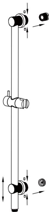
4. Push shower rail assembly onto the wall/tile face. Tighten grub screws firmly. Slide the back plates against the wall/tile face properly.
