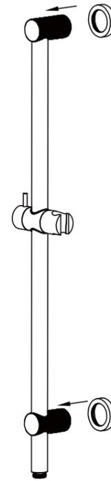
3. Slide both top and bottom back plate onto the rail assembly, as shown on the picture.
