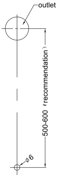
1. Drill a  $\phi 6$ mm hole at the downwards outlet vertical downward position in the recommended range.
