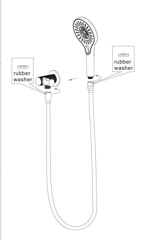
4. Connect bracket and hand shower with hose. TEST & CHECK FOR LEAKS.
