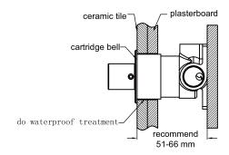
2. Put cartridge bell onto body and do waterproof treatment for the gap between cartridge bell and plasterboard and ceramic tile.
