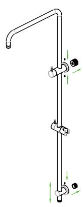
4. Locate and push shower rail assembly onto wall adaptors. Tighten grub screws firmly with allen key provided.
