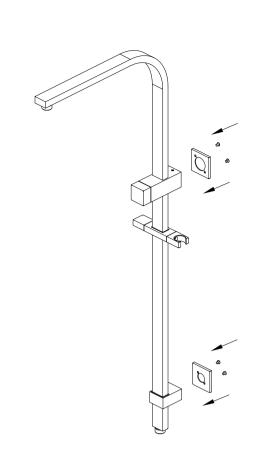
3. Screw the straight tube (with lower body) on diverter body, and then pull on the 2 dressing rings for both the diverter body and lower body.
