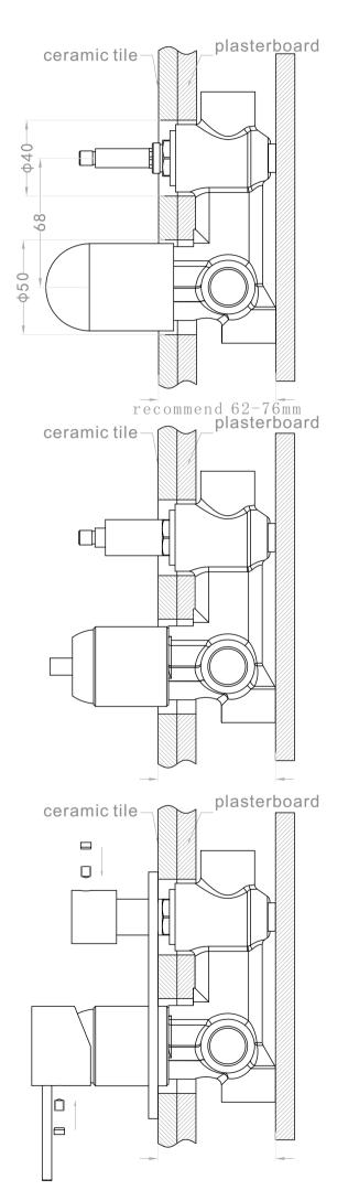
1. Fix body on noggin and ensure installation depth is 62-76mm from noggin to ceramic tile.
