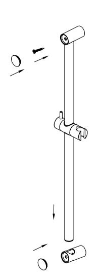
6. Plug shower rail in bottom bracket. Mount top bracket on the top hole by expansion plug and tapping screw. Push plates onto two brackets.
