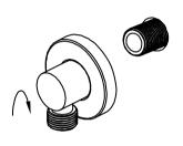
Screw elbow body on to outlet.
