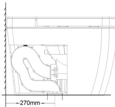
Water Pressure:0.15MPa-0.75MPa(dynamic pressure 1.5-static pressure 7.5kg) minimum flowrate is 5L/15s.
