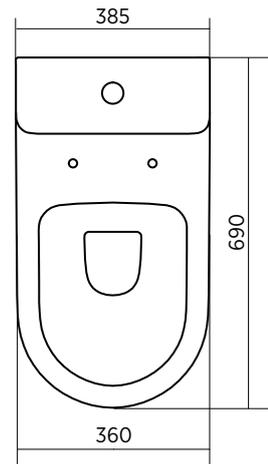
Rimless Clean Flush pan - for an efficient, powerful flush. Nanoglaze surface - ultra-smooth, anti-bacterial, easy to clean. Easy care height - making it easier to get on and off the seat.
